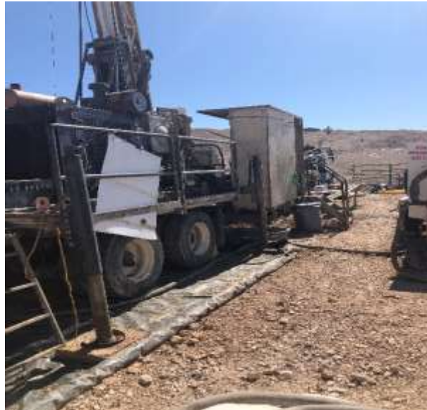
Figure 11-1: Truck Mounted Core Rig
